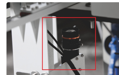
三个识别系统精准定位松紧带缝纫 Three-Sensor System for Precision Elastic Band Sewing
