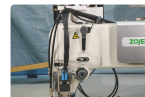
光电检测断线感应 Photoelectric detection for thread breakage induction
